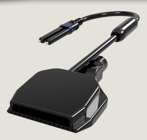
The DD 209 and DD 209 (A) discharging nozzles are flow-optimised. A greater electrostatic discharge reach and cleaning effect on the material to be discharged may be achieved with the additional support of compressed air. Air connection is provided via a G1/4" female thread.
