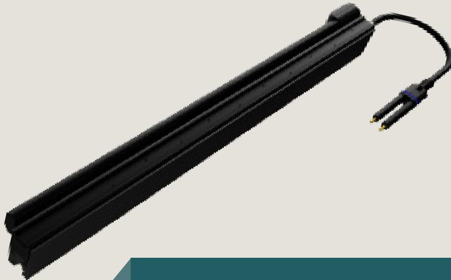
The DE 406 L is a highly stable universal electrode for a variety of applications. The stable aluminium profile design renders it suitable for longer self-supporting distances. A greater electrostatic discharge reach and material cleaning effect may be achieved with the additional support of compressed air.
